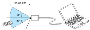
Remote sensor on the remote mouse receiver
